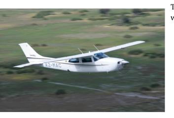
The *Cessna C210* centurion possesses a similar interior layout to that of the C206, it seats five passengers and with its retractable undercarriage, cruises at a comfortable 270 km/h and possesses a range of 1,485 km.
